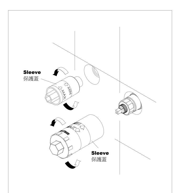
\* Remove **Sleeves** after complete Finished Wall, and then go for next steps.
