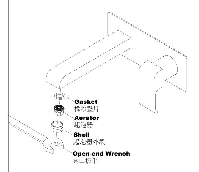
\* When finished installion, please disassemble the **Aerator** and **Gasket** counterclockwise with **Open-end Wrench**. (Please help to use the soft cloth to protect the Aerator Shell.)
