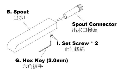
\* Loosen the **Set Screw** from **Spout** with **Hex Key(2.0mm)**, and disassemble the **Spout Connector**.
