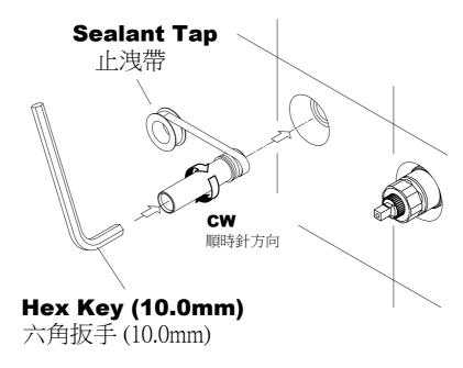
\* Apply pipe compound or thread sealant tape to the thread of **Spout Connector**, and screw the **Spout Connector** to the **Valve Body**with **Hex Key(10.0mm)**
