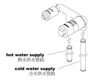
\* Install hot and cold water supply pipes as figure shows.
