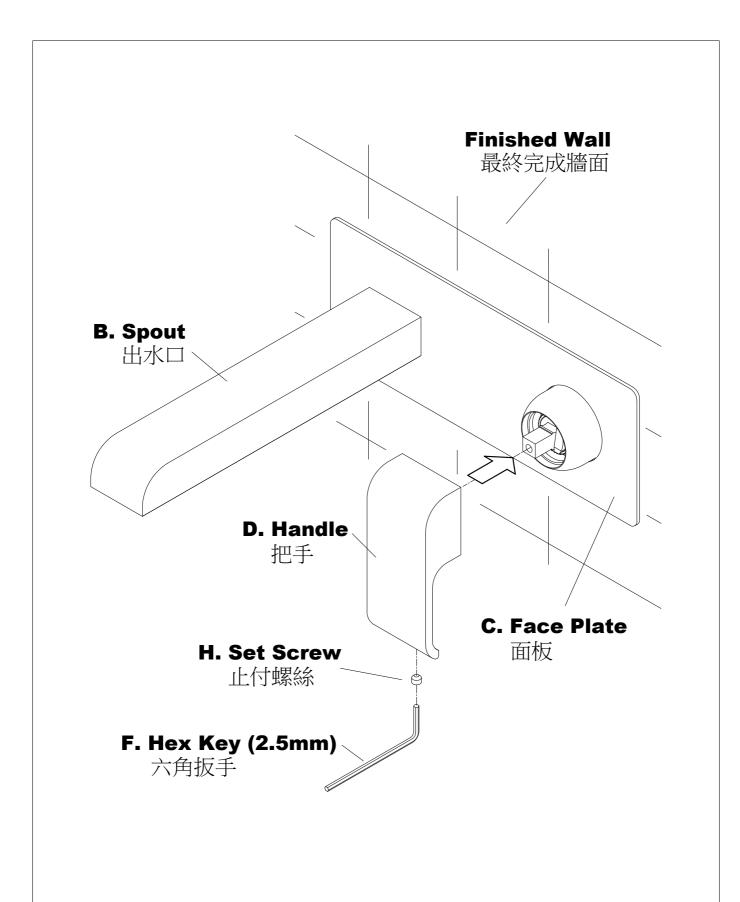
\* Fix the **Handle** to the Cartridge side of Valve Body with **Hex Key(2.5mm)**.
