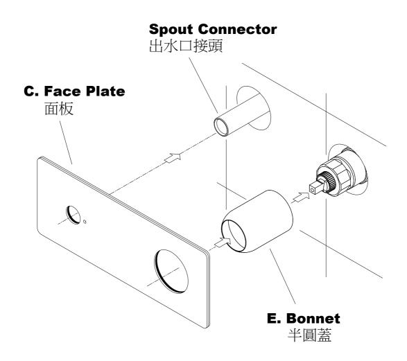
\* Cover **Bonnet** to the **Valve Body**. Install the **Face Plate** to be flush with **Finished Wall**
