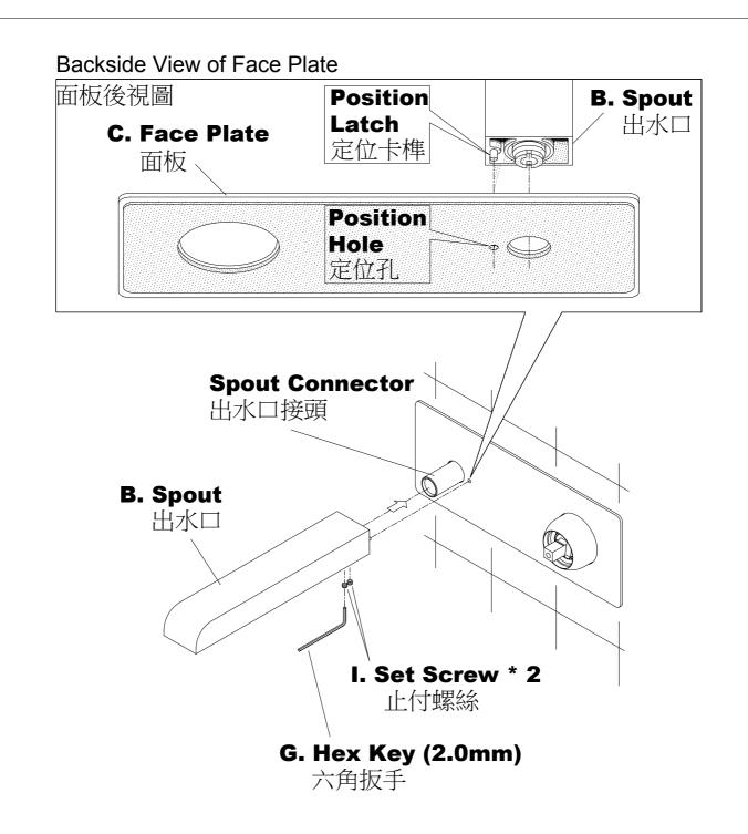
\* Aim the Position Latch of Spout at the Position Hole of Face Plate and insert the Spout Connector into Spout to make Spout be flush with Face Plate; tighten the Set Screw underheath Spout with Hex Key(2.0mm) to finish the installation of Spout.
