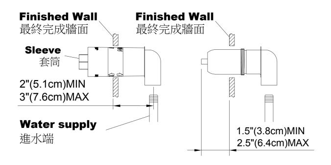
\* Connect hot and cold supply pipes to the **Valve Body**, and keep the distance between 2" (5.1cm) minimum and 3" (7.6cm) maximum from the Finished Wall to the center of **Valve Body**; or keep the distance be 1.5 " (3.8cm) to 2.5" (6.4cm) between top of cartridge and Finished Wall for necessary conditions.
